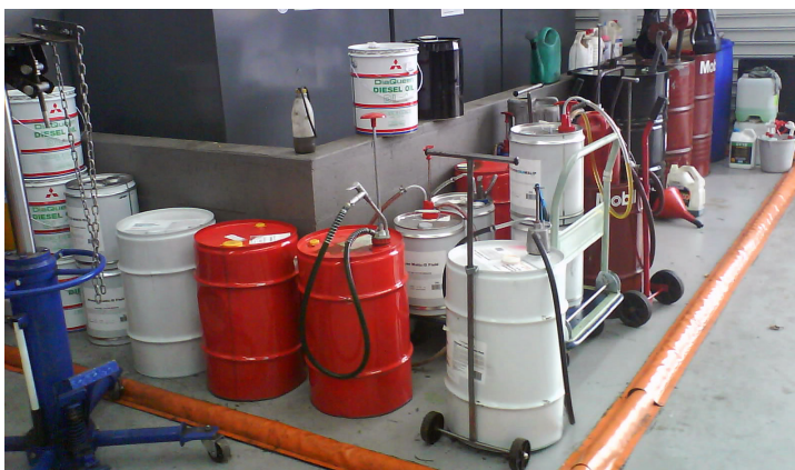
Two types of bunds can be seen in this picture: a bund for the bulk oils and a floor bund.
